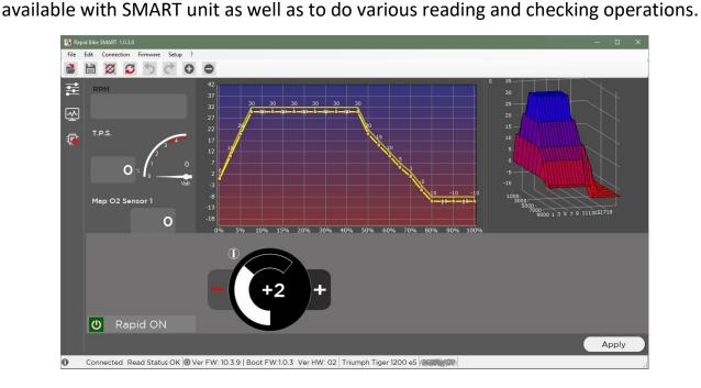
To connect with the SMART control unit, you only need an internal or external Bluetooth adapter to the PC at least release **4.0 BLE**. More information on the "Rapid Bike SMART" software manual, available with its installation.
